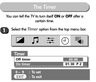
Select the **On timer** (or the **Off timer**). If, for example, you want the TV to turn ON (or OFF) in one and a half hours time, enter 01:30 using the numbered buttons on the remote control.
